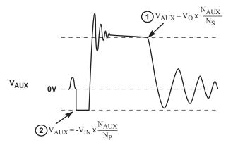
Figure 9.3: Auxiliary Voltage Waveforms
