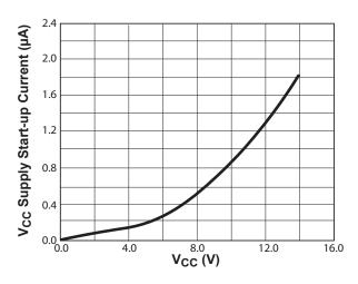
Notes: Figure 7.5 : V<sub>cc</sub> Supply Start-up Current vs. V<sub>cc</sub>
