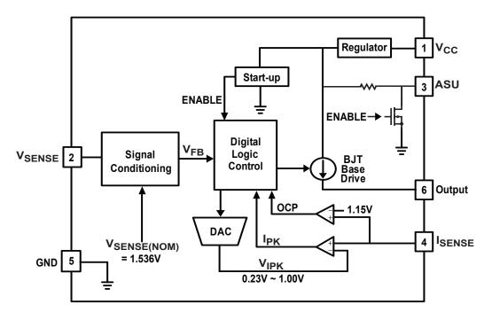
Figure 8.1 : iW1679-50 Functional Block Diagram
