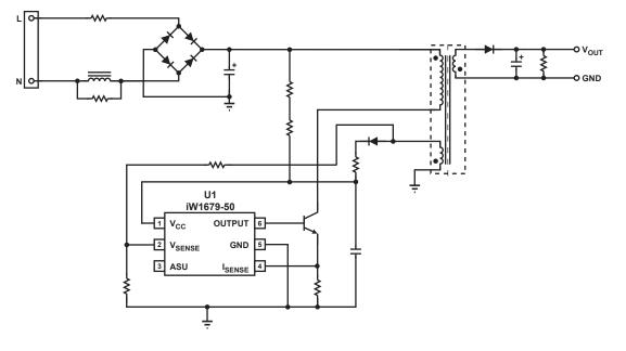
Figure 3.2: iW1679-50 Typical Application Circuit
