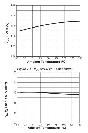
Figure 7.3 : Switching Frequency vs. Temperature<sup>1</sup>
