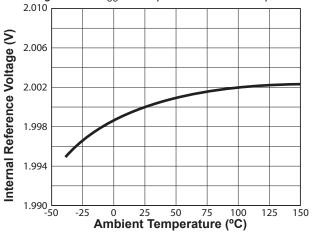
Figure 7.4 : Internal Reference Voltage vs. Temperature
